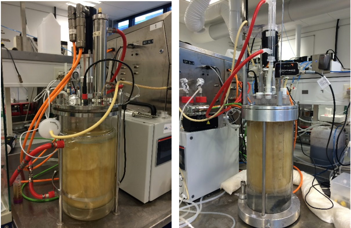
One glass/steel STR and one BactoVessel SUF both liquid cooled and connected to the twin channel Biostat PCS with liquid thermal control. SUF installed in a Re-Usable-Jacket for efficient heat transfer. Two independent servo motor drives in order to reach the 2000 RPM target. Photo by Per Stobbe.
