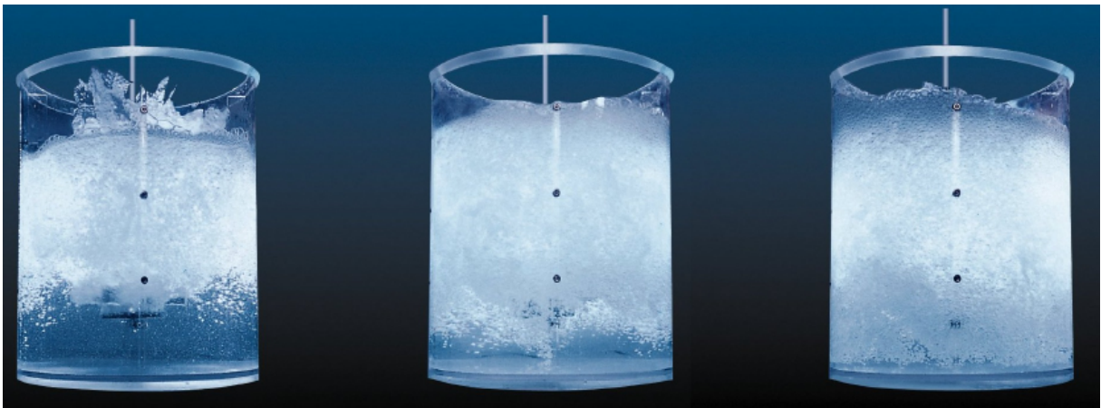
Photo 1 illustrate visual inspection the mixing gradients, differences. Flat blade Rushton left being the worst, Smith middle significant better and Bakker right even slightly better. Photo by André Bakker.
