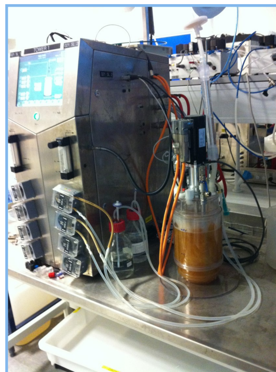
3 Liter Single-Use fermenter (SUF) running a fermentation with E. coli.
