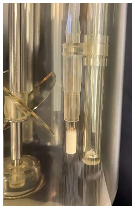
FIGURE 2 Integrated frit sparger as developed for CerCell® 3 L single-use bioreactor (CerCell A/S, Denmark).
