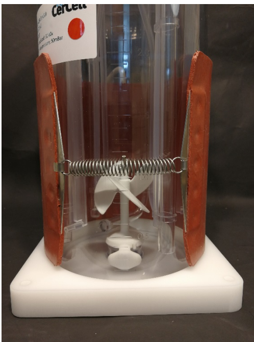
Photo left: Stretching the small springs to 50 – 60 % longer than standard and seek to obtain the in total 3 kilo / 30 Nm clamping force. Use extra springs or any metal, plastic ring to obtain the required clamping force.
