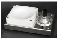
All MST facilitate as an extra a square block with selectable ID centring foot for precise and stable mounting of the SUB, SUF, SUM and various spinner flasks. Able to handle the elevated temperature like 37°C in controlled environment.
