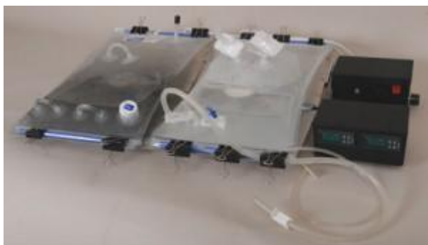
Figure 5. Cultivation systems used. CerCell's CellTumbler platform fitted with 2x5L Cell Bags. Note that the transfection experiment was performed in 1L scale in 2L cell bags.
