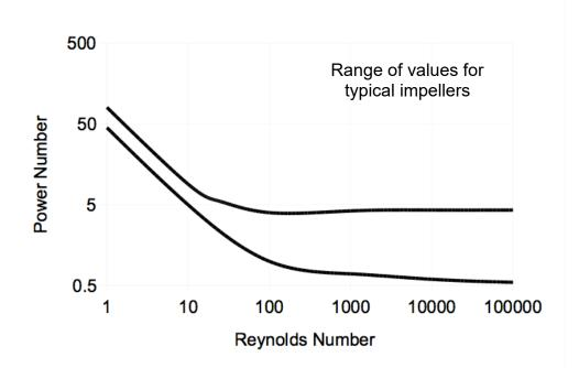
Power Number as a function of Reynolds number for a range of typical impellers.
