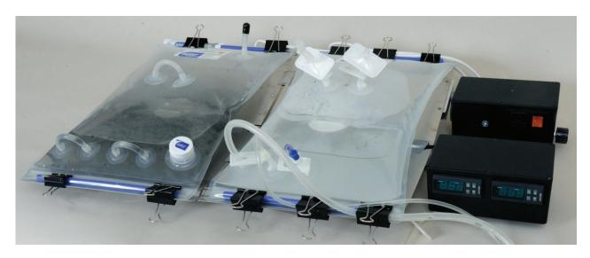
Any commercial available wave bag up to 10/20 litre may be used and operated independtly with temperature and gas control.
