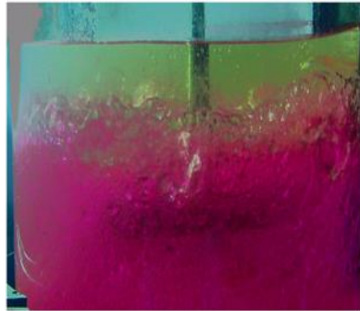
Photograph showing the cylindrical vessel in operation with straight bladed impeller small size (Impeller no. 1) at higher rpm (94rpm) and it can be observed that inter dispersion between the phases is reduced due to increased turbulence.
