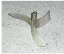
Tiltation angle = 20^\circ Power required with impeller # 3
