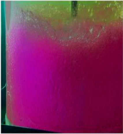
Photograph showing the cylindrical vessel in operation with 12 degree curved impeller blades (Impeller no. 4) at lower rpm (77rpm)
