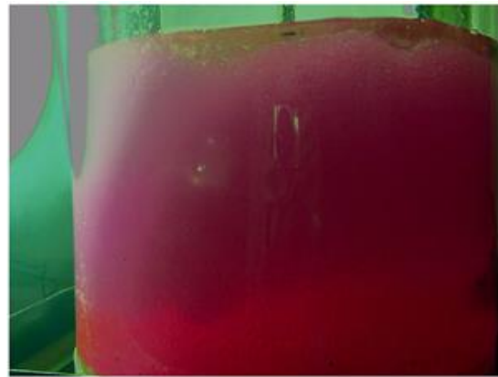
Photograph showing the cylindrical vessel in operation with straight bladed impeller large size (Impeller no. 2) at lower rpm (55rpm) and it can be observed that emulsification is created between the phases. The flow patterns can be observed, drop size is smaller
